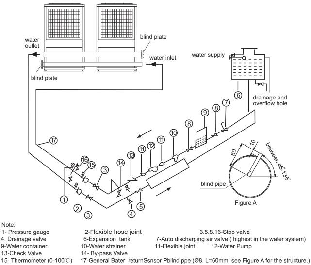
When cycle water runs for the first time, close the inlet/outlet valve (No. 3) and open the by-pass valve (No.14). When water pump works for a while, clean the water strainer. After confirming that there is no impurity in the external cycle system, open inlet/outlet valve (No. 3) and close the by-pass valve (No.14). Then, the unit is in normal operation.
